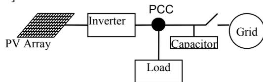
Figure 9: System configuration
