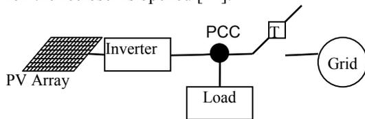
Figure 7: System configuration
