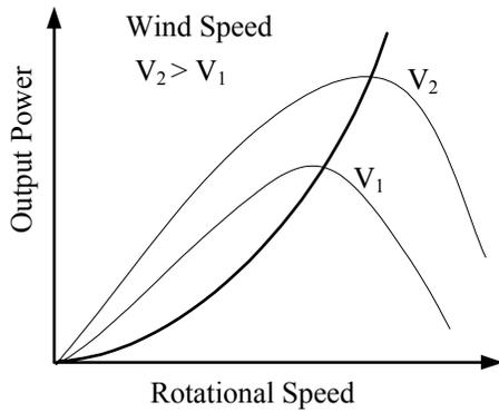
Fig.2. Relationship between the generator output power and rotational speed.
