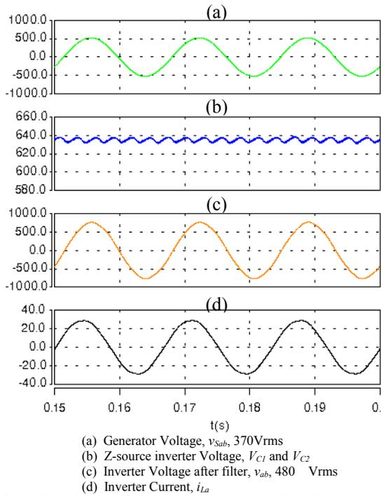
Fig.6. Simulation waveforms when the generator voltage is 370 Vrms, 15 kW with boost mode control.
