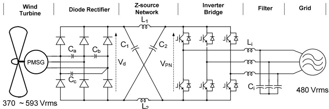
Fig.4. Proposed Z-source inverter for the wind power system.
