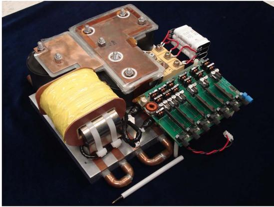
Fig. 8. A 10 kW Z-source inverter for Wind Power System
