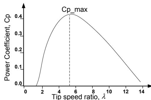
Fig. 1. Curve showing variation of the power coefficient of performance with the tip speed ratio.
