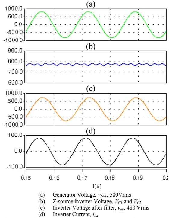
Fig.7. Simulation waveforms when the generator voltage is 580 Vrms, 45 kW without boost condition.
