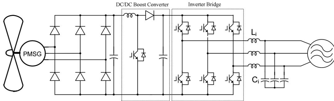
Fig.3. Conventional Inverter with DC/DC Boost Converter for the wind power system.
