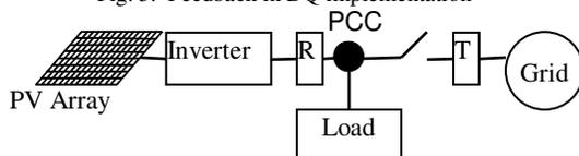
Fig. 6. System configuration including
