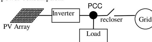
Fig. 1. System configuration
