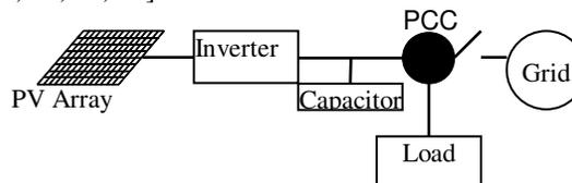
Fig. 2. System configuration
