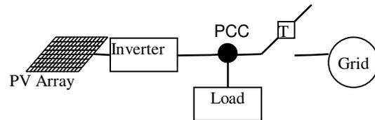
Fig.7. System configuration
