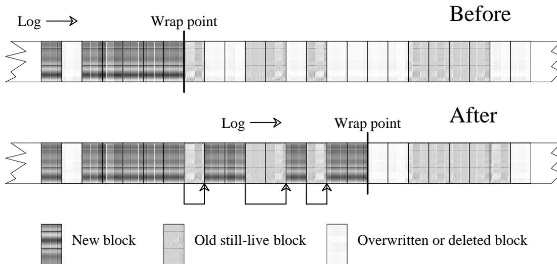
**Figure 4-2 — A threaded log-structured file system**
