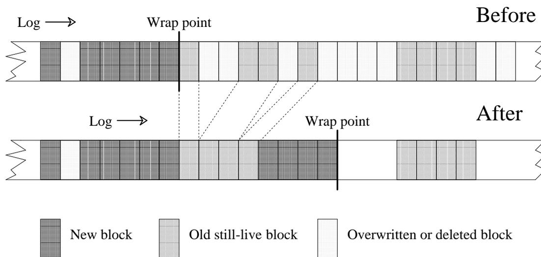
**Figure 4-3 — A copying log-structured file system**
