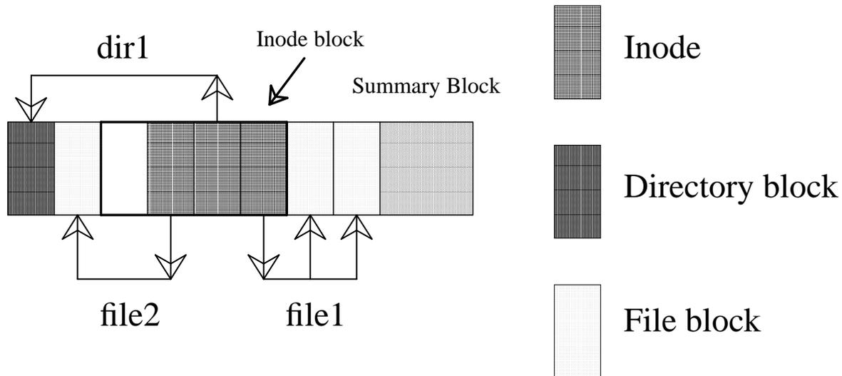
**Figure 4-5 — Layout of a Sprite LFS log region**
