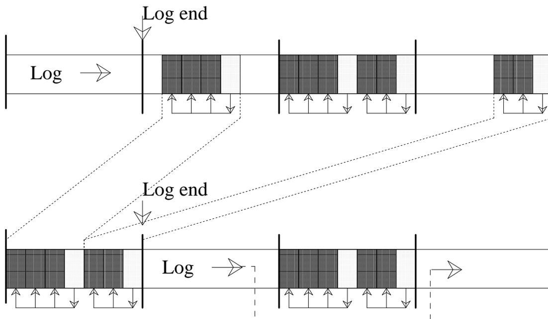
**Figure 4-4 — Segment cleaning in Sprite LFS**
